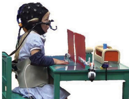
Fig. 4. Simultaneous, real-time capture of video, motion-tracking data, eye-tracking data, and EEG (Ossmy et al., 2022).
